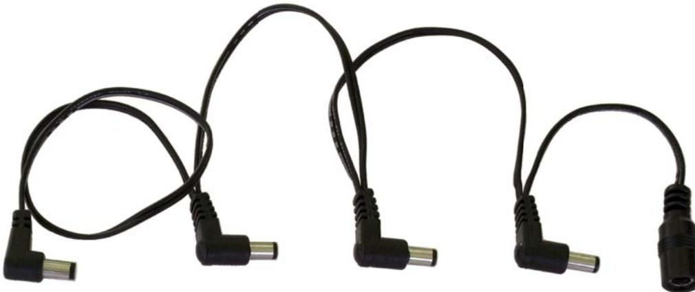
If you have several stompboxes powered with direct current (DC) and the same voltage, you can connect them to a single power supply using the 5-plugs distribution-cable. All effects together must not consume more current (mA) than specified at the power jack of the XDS. If you do not need all five plug, isolate the unused ones with insulating tape!
